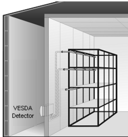
Figure 5– Example of in-rack air sampling.
